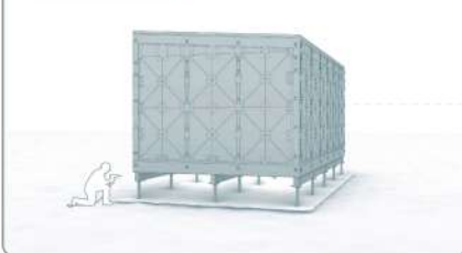
Fix Vertical Cladding to Cavity Battens
