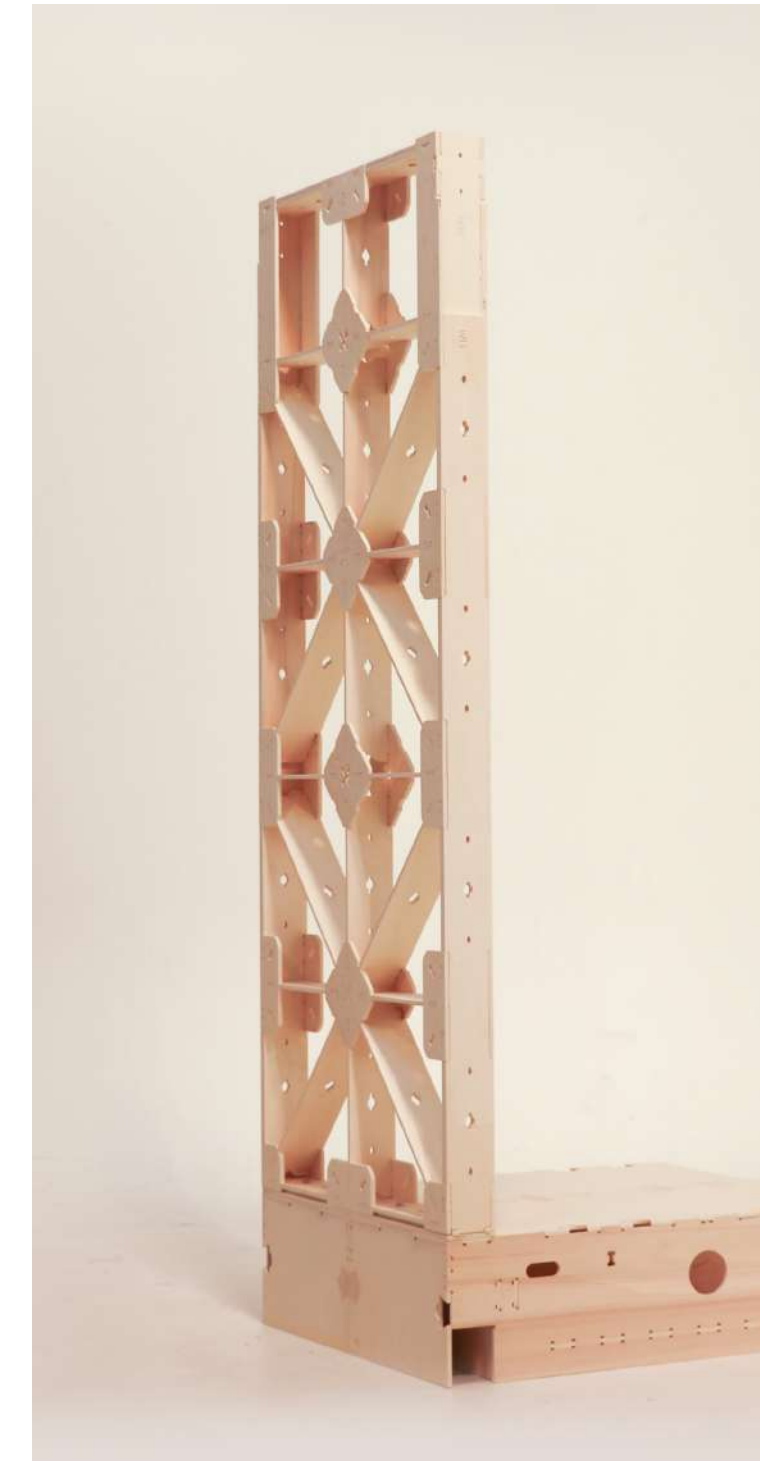
1:2 Physical Model WikiHouse Floor Block (SKYLARK250-XS) + XFrame Wall (2700mm) Prefabricated Plywood System Test
