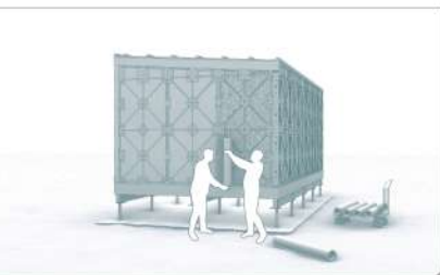
Weather Resistive Wrap around structure
