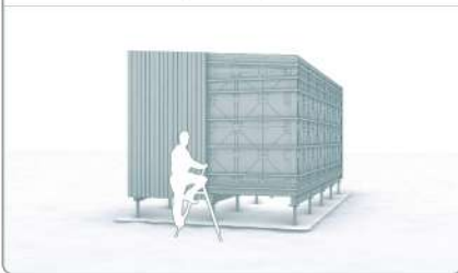
Fix Vertical Cladding to Cavity Battens
